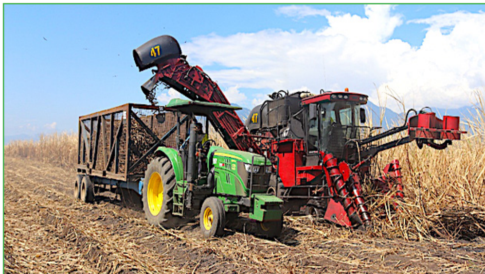
A sugarcane harvester cutting and loading harvested canes onto a tractor trailer for transportation to the main factory at Gusap
